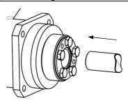
Push in the shaft (h6) at least to the minimum fitting length (see data sheet). Caution: The tensioning screws of the shrink disc may not be tightened as long as there is no shaft in the gearbox's hollow shaft. Tightening the tensioning screws without a shaft would deform the gearbox's hollow shaft.
