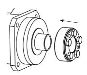
Pushing the shrink disc onto the gearbox's hollow shaft.
