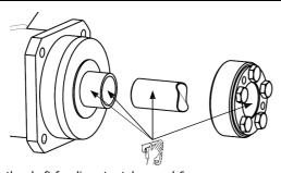
Check the shaft for diameter tolerance h6. Clean the components free of grease as shown in the figure. 4.
