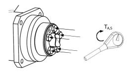
Tighten the shrink disc's tensioning screws evenly in stages one after the other in several circuits up to the maximum permitted tightening torque  $T_{A.S.}$
