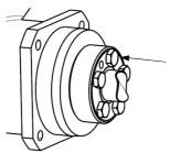
Check whether the front surfaces of the outer and inner rings are aligned. Only when this is the case, has the correct tightening state of the shrinkage disk been achieved. It is recommended to check all tensioning screws one after the other twice with maximum tightening torque  $T_{A,S}$ .
